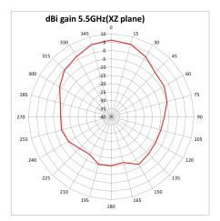
Radiation Pattern for 5GHz Antenna 2
